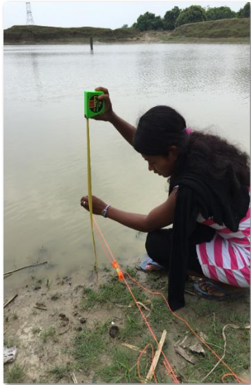
Figure 9 Measuring the depth of water in a pond using a spirit level, stringline and a tape measure
