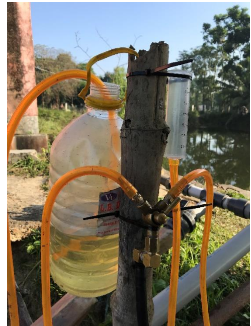
Figure 11 A brass 3-way valve used to supply 50ml (from a syringe) of diesel to a pump
