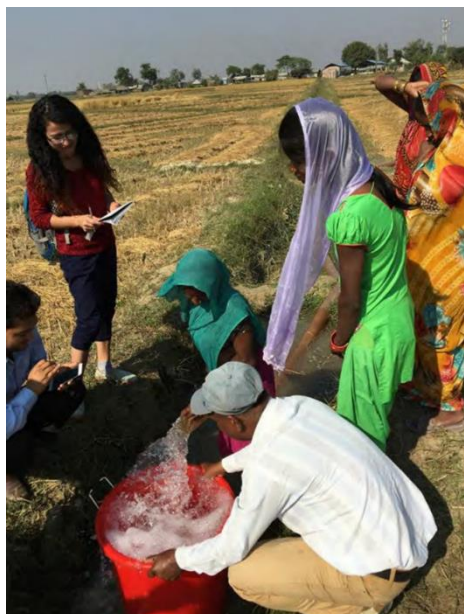
Figure 34 Using a bucket and stopwatch to measure flowrate for pump assessments
