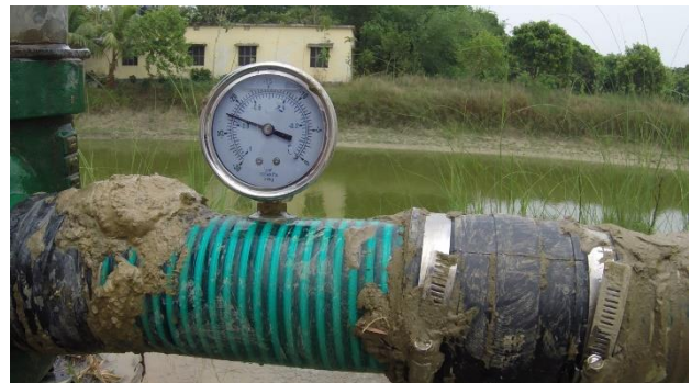
Figure 13 Ensuring air tight seals is needed to collect accurate pressure readings
