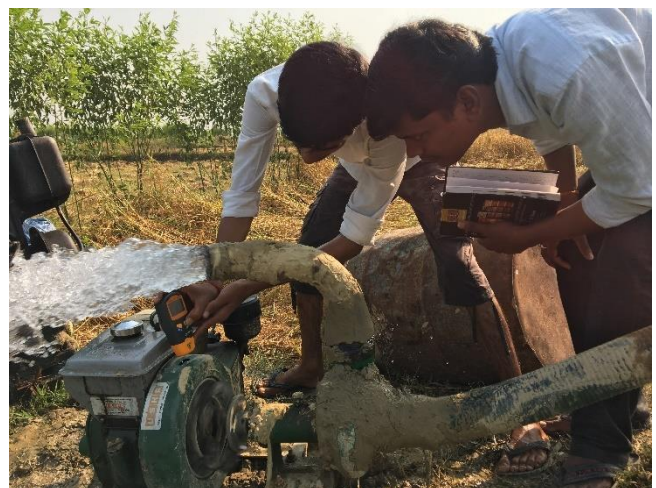
Figure 12 Field staff using a digital tachometer to measure the pump speed (RPM) to find the Best Efficiency Point
