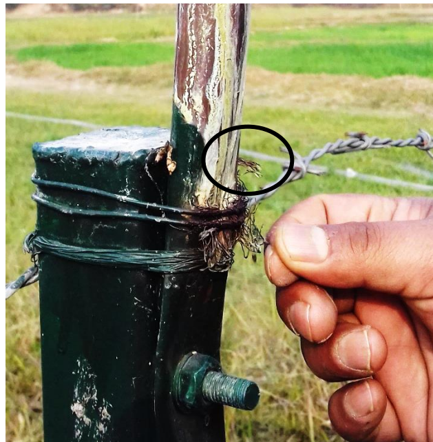
Figure 16: Broken Earthing Wire
